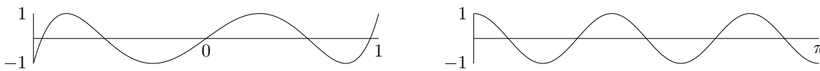
Figure 1: Comparison of the Chebyshev polynomial T_5(x) on the left with \cos 5\theta on the right.
